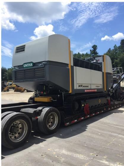
The world-renowned shredding technology has made the 4,700-mile journey from UNTHA's manufacturing hub in Salzburg, to Geocycle's 13-acre site in Dorchester, SC. Here, the mobile unit with 2 x 177hp motors, will process non-hazardous post-industrial waste to produce a <3" RDF fuel that will be used for energy recovery in the nearby Holly Hill cement plant.
